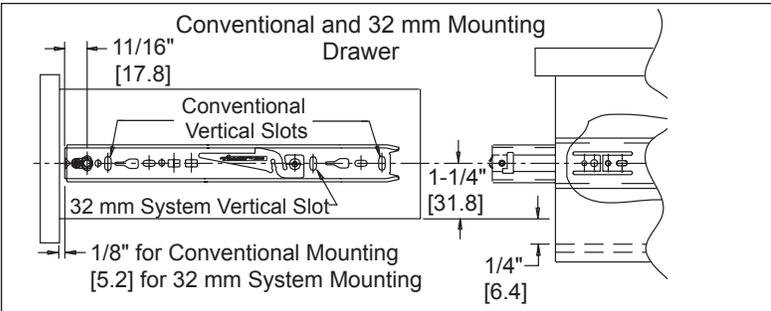
4. Make sure the ball bearing retainers in the cabinet side are fully forward. Install drawer into cabinet. Close the drawer.
