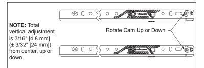
5. **IMPORTANT:** After all adjustments are made, secure rail with additional mounting screws.
